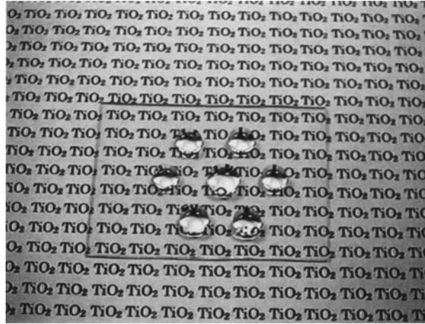
Fig. 2. Transparent super-hydrophobic thin film with \text{TiO}_2 photocatalyst
